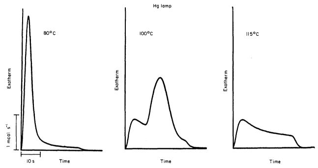
Figure 2 Exotherms of F12H10MA initiated with unfiltered medium-pressure mercury lamp at (a) 80°C, (b) 100°C and (c) 115°C
