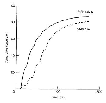
Figure 7 Cumulative percentage conversion versus time plots for F12H10MA and CMA-10 ( $\lambda_{ex}$  = 351 nm; pulses 15 s apart; 1.19 mJ cm<sup>-2</sup> pulse<sup>-1</sup>) generated with pulsed excimer laser
