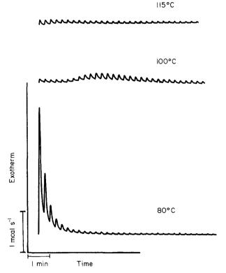
Figure 5 Single-pulse exotherms of F12H10MA at (a) 80°C, (b) 100°C, and (c) 115°C initiated with pulsed excimer laser ( $\lambda_{ex} = 351$  nm; pulses 15 s apart; 4.17 mJ cm<sup>-2</sup> pulse<sup>-1</sup>)
