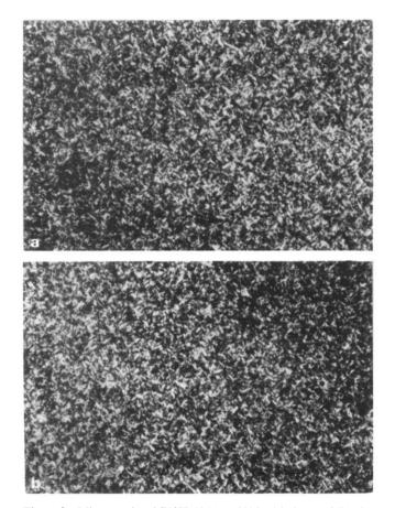
Figure 3 Micrographs of F12H10MA at 80°C (a) before and (b) after polymerization by exposure to the output of a medium-pressure mercury lamp
