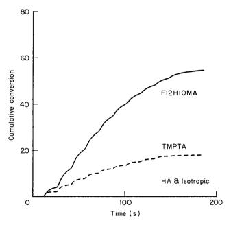
Figure 8 Cumulative percentage conversion versus time plots for F12H10MA at 80°C and 100°C, TMPTA, and HA ( $\lambda_{ex}$  = 351 nm; pulses 15 s apart; 0.11 mJ cm<sup>-2</sup> pulse<sup>-1</sup>) generated with pulsed excimer laser
