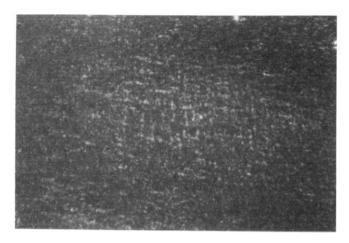
Figure 4 Micrograph of F12H10MA at 100°C after polymerization by exposure to a medium-pressure mercury lamp
