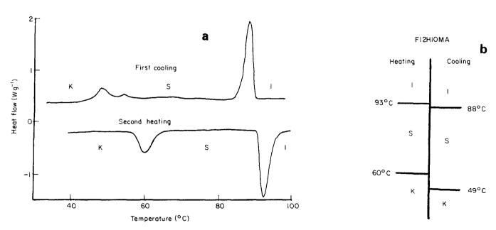
Figure 1 (a) First d.s.c. cooling cycle and second d.s.c. heating cycle for F12H10MA and (b) pictorial of d.s.c./optical microscopic examination of F12H10MA (K=crystalline; S=smectic; I=isotropic phase)
